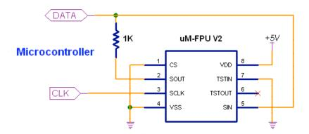
If a 2-wire SPI interface is used, the SOUT and SIN pins should not be connected directly together, *they must be connected through a 1K resistor*. The microcontroller data pin is connected to the SIN pin. See the uM-FPU datasheet for further description of the SPI interface.
